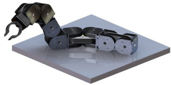
Fig. 16. A serpentine assembly of iMobot modules with a gripper [91].
