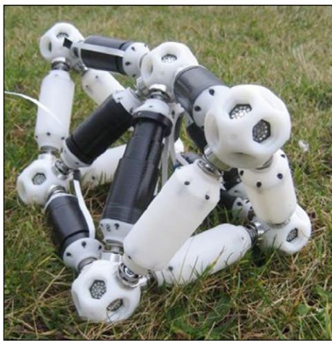
Fig. 10. A lattice assembly of links and joints for the Odin modular robot [59].
