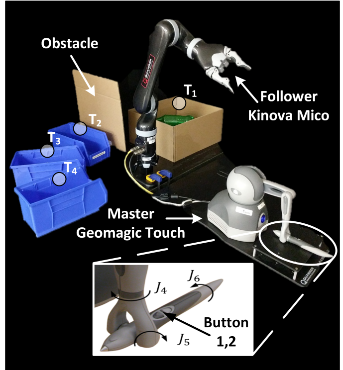
FIGURE 3: Experimental setup with indicated master and follower systems, environmental obstacles, and operational targets (T1-T4).
