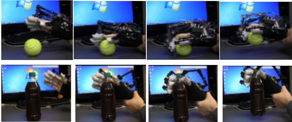
Figure 9: Wooden hand executing manipulation tasks. Top row: the wooden hand approached the tennis ball (by the author), grasped it, and lifted it (by the author) from the table. Bottom row: the wooden hand was controlled to grasp a bottle of water. The whole procedure setting was similar to the tennis ball grasping.
