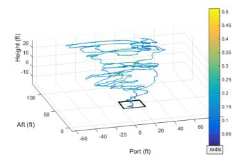
Figure 10. Isometric view of the ship air wake intensity plotted on the helicopter's trajectory.
