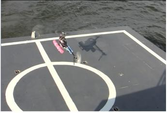
Figure 3. Rover module mounted on helicopter approaching flight deck of Modified YP676 vessel
