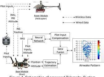
Figure 4. Schematics of proposed Telemetry System
