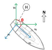
Figure 9. Coordinate system of the ship
